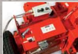
Cut length adjustment (12 lengths) through 4-speed gearbox, electrical operating panel from the driver's cab.
