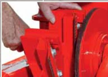
The sharpening stone allows the blades to be sharpened easily and reliably.
