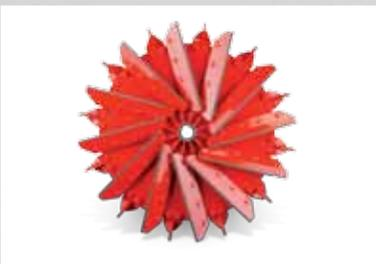
All mounted forage harvesters include a powerful flywheel. The blade holders support grain cracking. The flywheel can be adjusted towards the counter-blade.
