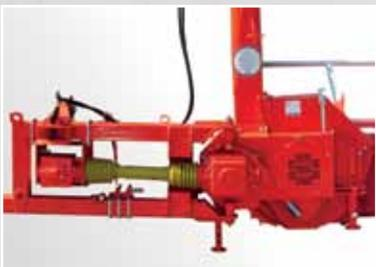
The mounting frame for front, side and rear fitting.
