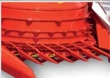
Intake drums with aggressive teeth ensure that the crop is gathered without loss, even under extreme conditions.
