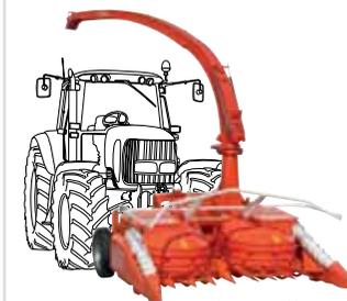
Front mounting with maize header
